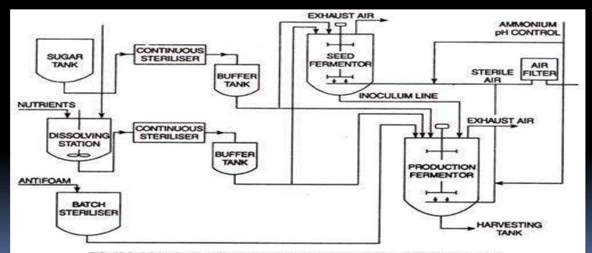
FIG. 40.6. A flow diagram of commercial production method of glutamic acid (glutamate).
